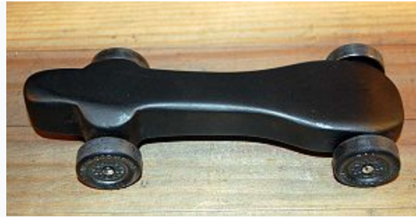
Bullet design with shaved and coned wheels, beveled and notched axles, and drilled axle holes.
